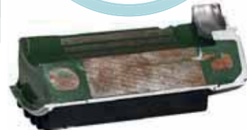
Insulated motor winding cross section
